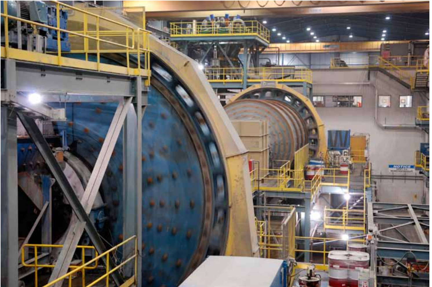
THINK BIG: The SAG Mill and Ball Mill at Agnico Eagle's Meadowbank mine in Nunavut. REUTERS/EUAN ROCHA
